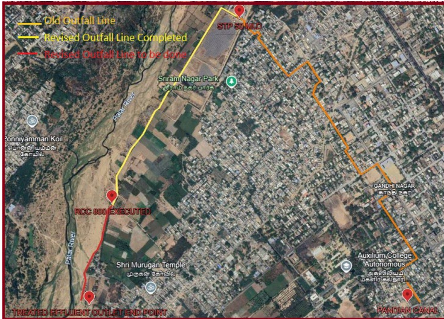
Figure 5: Revised Location of Outfall Sewer from Sewage Treatment Plant
